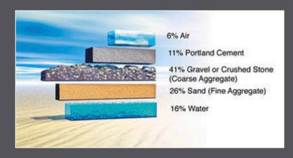
throughout the concrete. These tiny bubbles function as relief valves when water in the concrete freezes, helping to prevent surface deterioration. The typical air entrainment for exterior flatwork is in the five-to-seven percent range.
